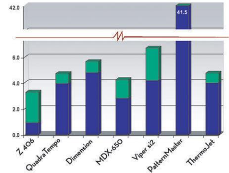
Chart 1..Average time for the complete prototyping process.
